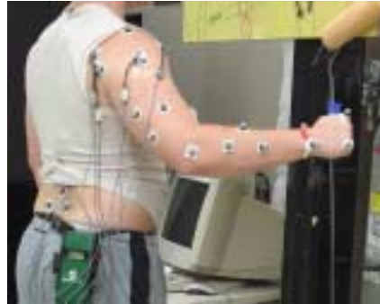
Figure 2: Surface Electrode and Reflective Marker Placements
